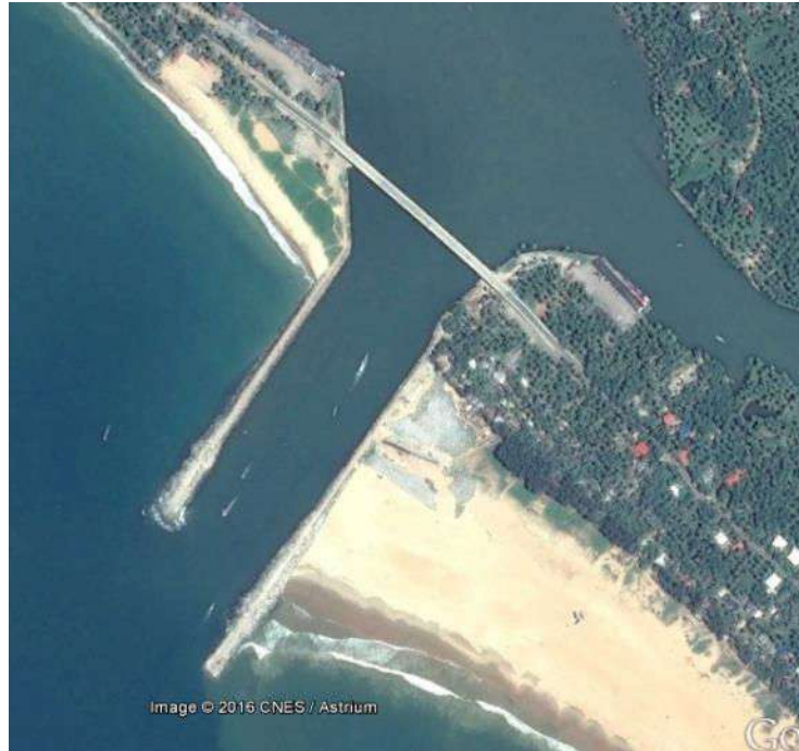
Fig. 5.4. Beach formation and erosion respectively on the south and north sides of harbour breakwaters at Muthalapuzhi
